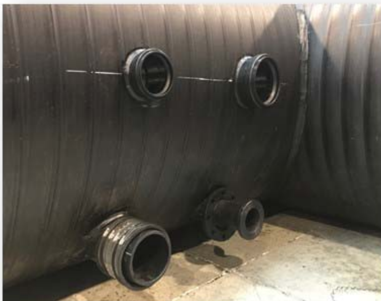
Figure 8 – Typologie de piquage
