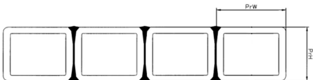
Figure 2 – Paroi de la buse TUBAOTEC
