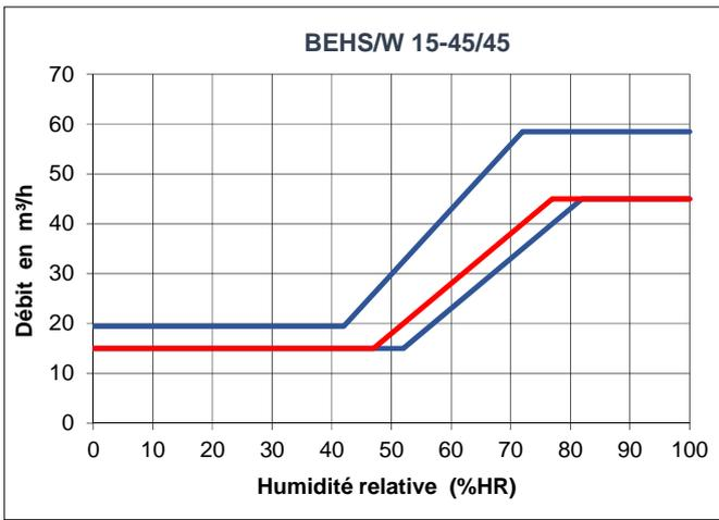
Figure 27 – HT05 et HV05 – BEHS/W ou BEHS/W.DP 15-45/45 (47-77%HR)
