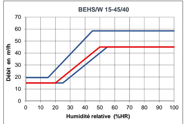
Figure 26 – HT04 et HV04 – BEHS/W ou BEHS/W.DP 15-45/40 (20-50%HR)
