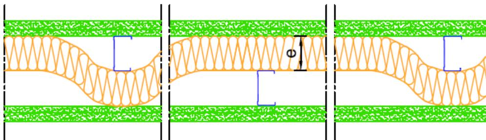
Figure 2 – Coupes horizontales - Cloison PREGYMETAL S/900 (Cf. article 5.54)
