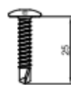
Vis PERFIX TORX PANEL 4,8x25 inox A2 et A4 support acier ou aluminium
