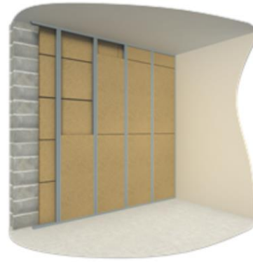
Figure 4-2: Insertion de la 2 e couche ISONAT FLEX (40mm) entre montants M48
