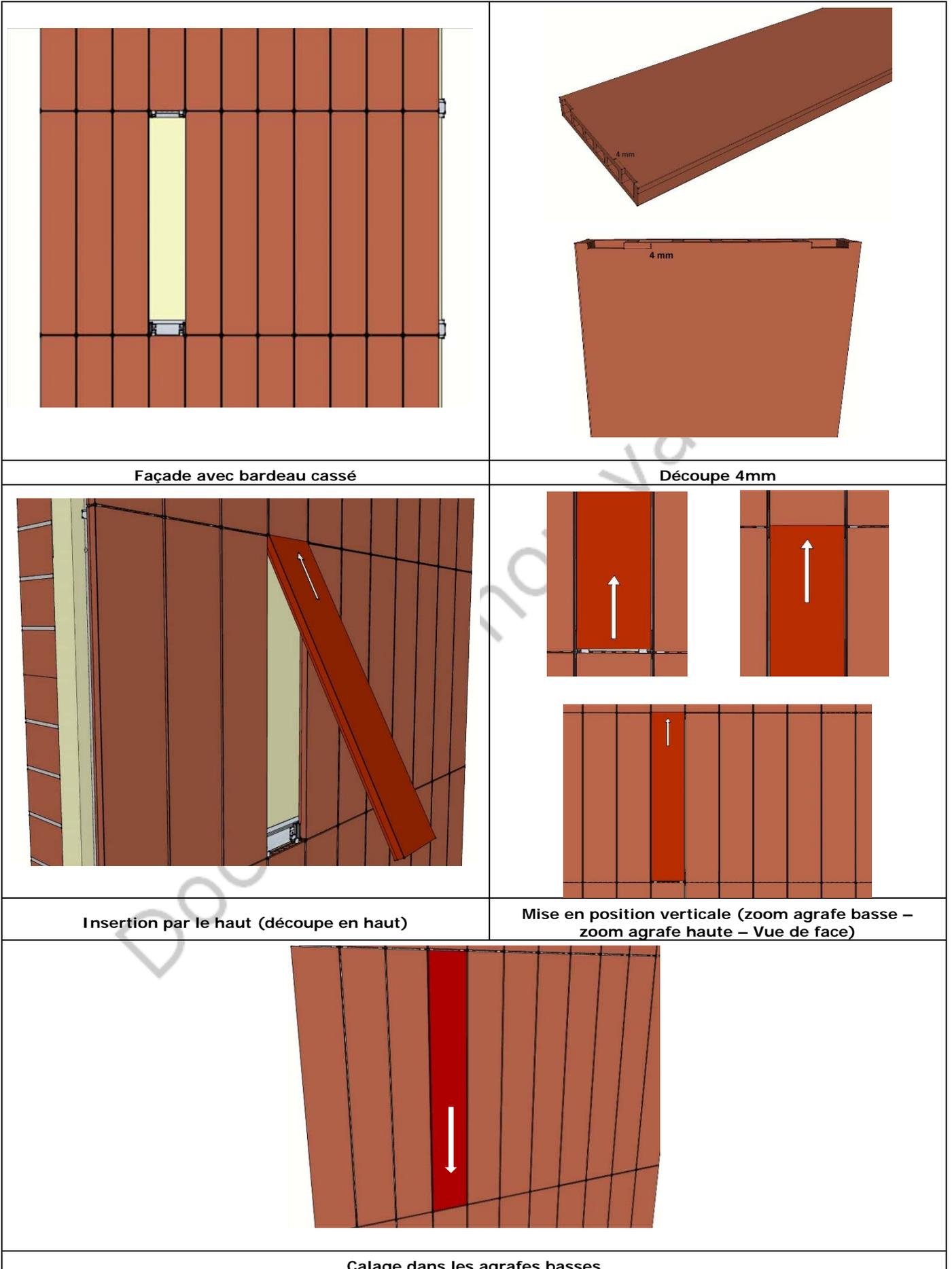
**Figure 14 – Pose renforcée**
