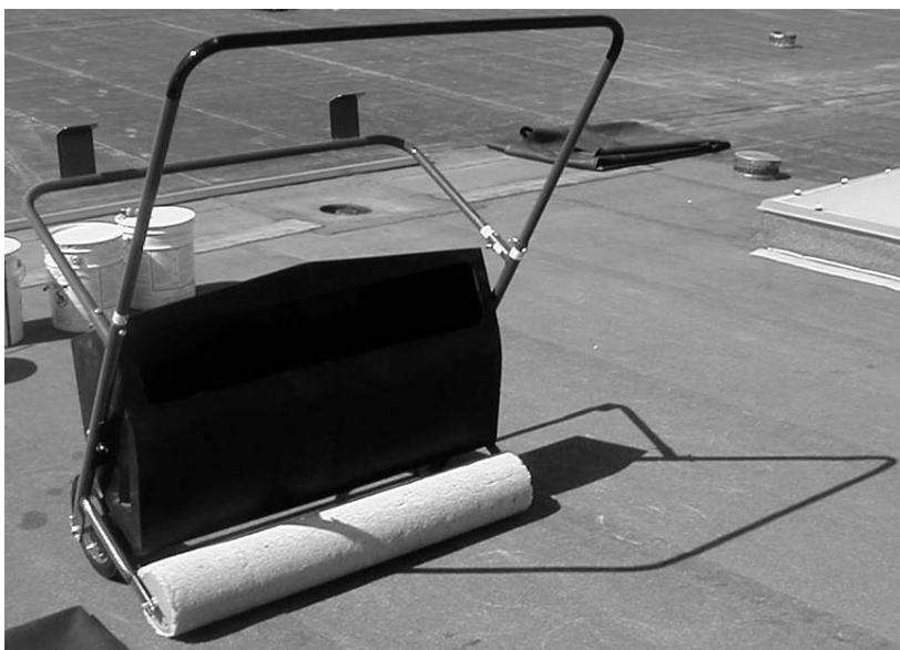
**Figure 19 – Machine SuperSpreader**
